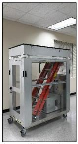
Position the mobile containment unit in the approximate location where ceiling access is required.
