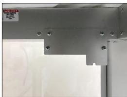
Locate the pressure monitor mounting bracket on the inside back wall of the AG8000.
