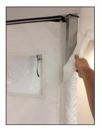
Both the top cover and the fabric enclosure are fastened to the mobile containment unit via hook and loop. To remove the top cover, simply separate the hook and loop along the perimeter of the top cover. To remove the fabric enclosure, detach the hook from the loop from each of the four telescoping members as shown above. Then separate the hook and loop along the top perimeter and then the bottom perimeter.
