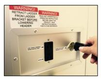
Power must be supplied to the AG8000 in order for any of the outlets to be operational. Plug the female end of an extension cord into the POWER SUPPLY outlet located on the back side of the unit and the male end into a 110V-120V, 60Hz, single phase outlet.
