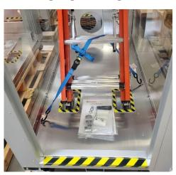
The AG8000 should be secured to ensure that the unit does not roll during transport and transported in its normal position (resting on its casters). If extremely poor road conditions exist, or excessive shock and vibration are expected, take precautionary measures by padding the unit to provide impact absorption during transport.
