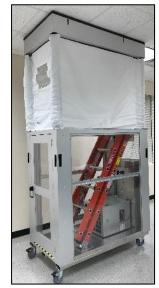
Raise the header within a few inches of the ceiling, ensuring that the unit can still be moved without crashing into any objects.
