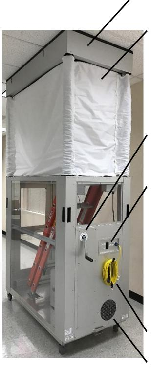
H. Header. The manual refers to this part as the header, which is raised and lowered using the provided hand crank or a power drill with clutch (not provided).
