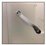
Turn hand crank clockwise to raise the header. Turn hand crank counter-clockwise to lower the header.
