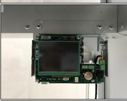
Remove the faceplate from the RPM series pressure monitor by unscrewing the two small screws on the sides of the pressure monitor. Connect the reducing elbow to the "COM" port of the monitor and attach tubing to the other side of the elbow. Plug the power connector into the terminal as shown. Hang the monitor on the lower set of screws on the mounting bracket.
