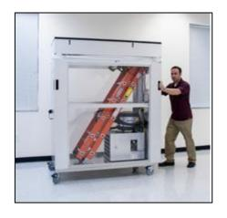
Transport the AG8000 in the fully collapsed position and use the handles located at the corners of the unit to move the mobile containment unit.
